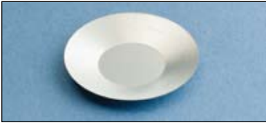
Fig. 17 Steel disk found inside the packaging box of welding material.
