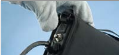
Fig. 26 Using the CADWELD EXOLON battery pack, press the button. At this time, the unit will send a charge to the igniter pin. The igniter pin will initiate the CADWELD EXOLON exothermic reaction. Allow approximately 30 seconds for completion of the reaction and solidification of the molten material.
